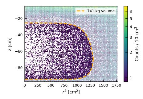
Super-ellipsoidal shape to reduce material backgrounds while maintaining large signal acceptance
