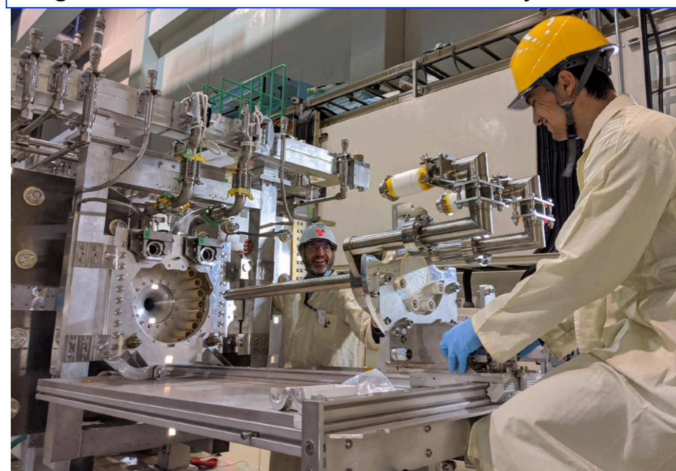
Target installation test to new Horn1 by RAL team
