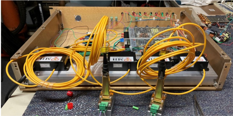
PoF - Power housing unit (5 warm Transmitter laser diodes)
