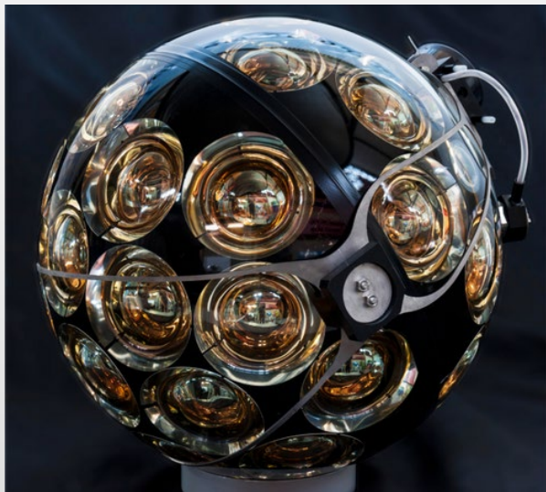
Digital Optical Module (DOM)
