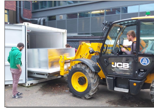
VIDARR Detector developed at the University of Liverpool, re-visit of supplementary Wylfa data underway (UK), 2D segmented, plastic scintillator
