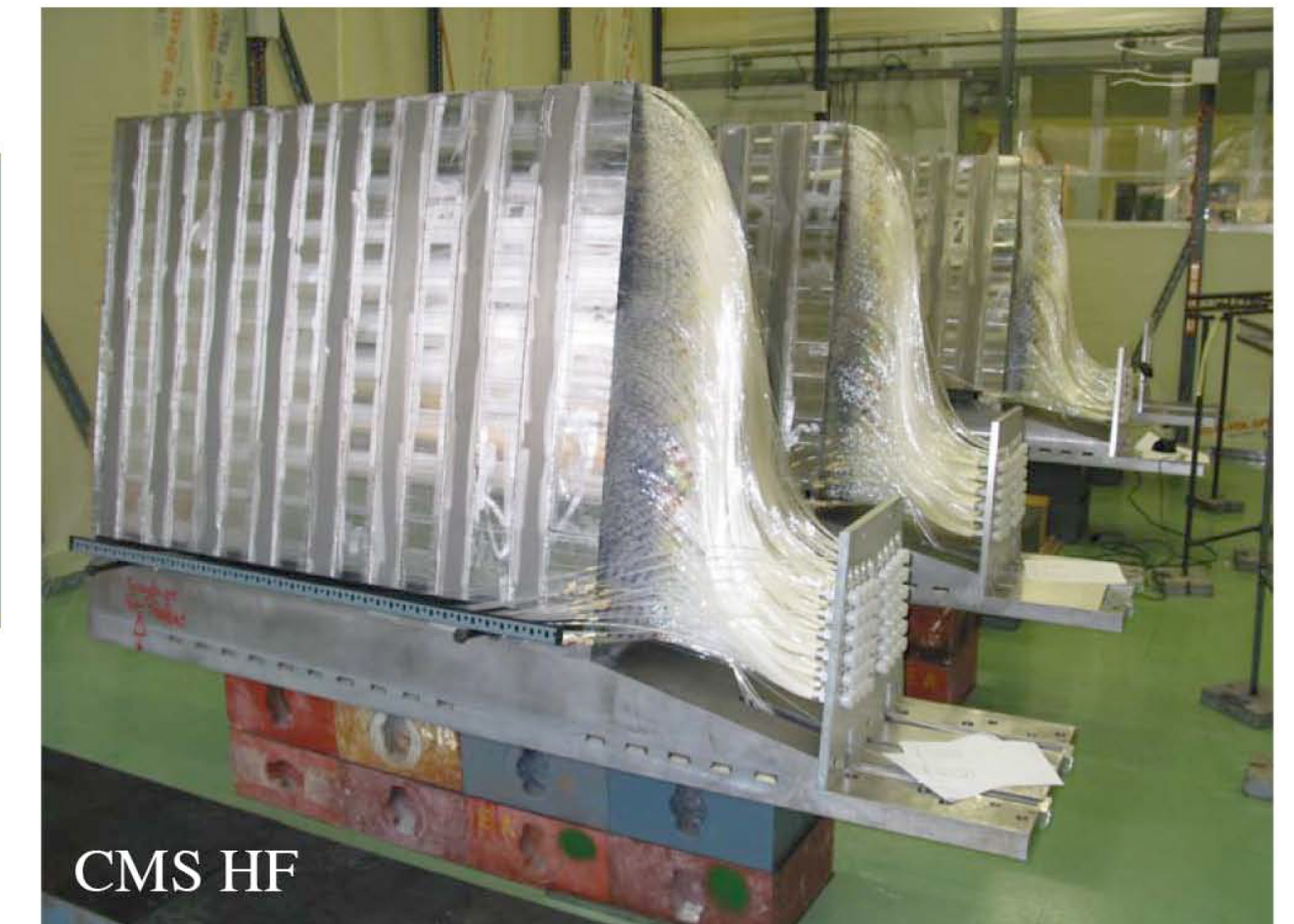
Figure 9.21: Schematic structure of a sampling calorimeter ( left ). Modules of the forward calorimeter of the CMS experiment ( right ).
