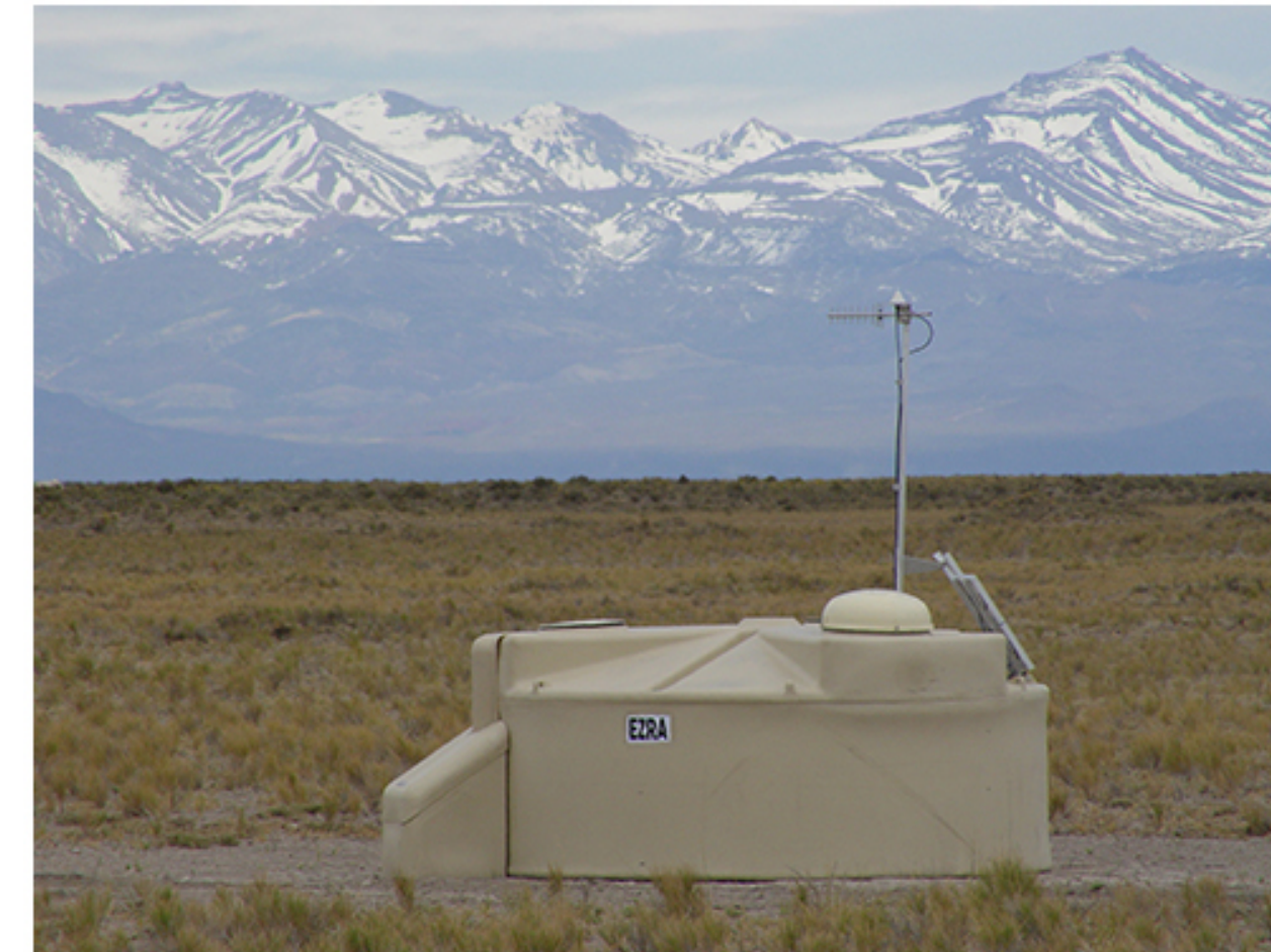
Figure 9.15: One of the more than 1600 detectors comprising the Auger experiment in Argentina, and the type of cosmic rays the experiment aims to detect.
