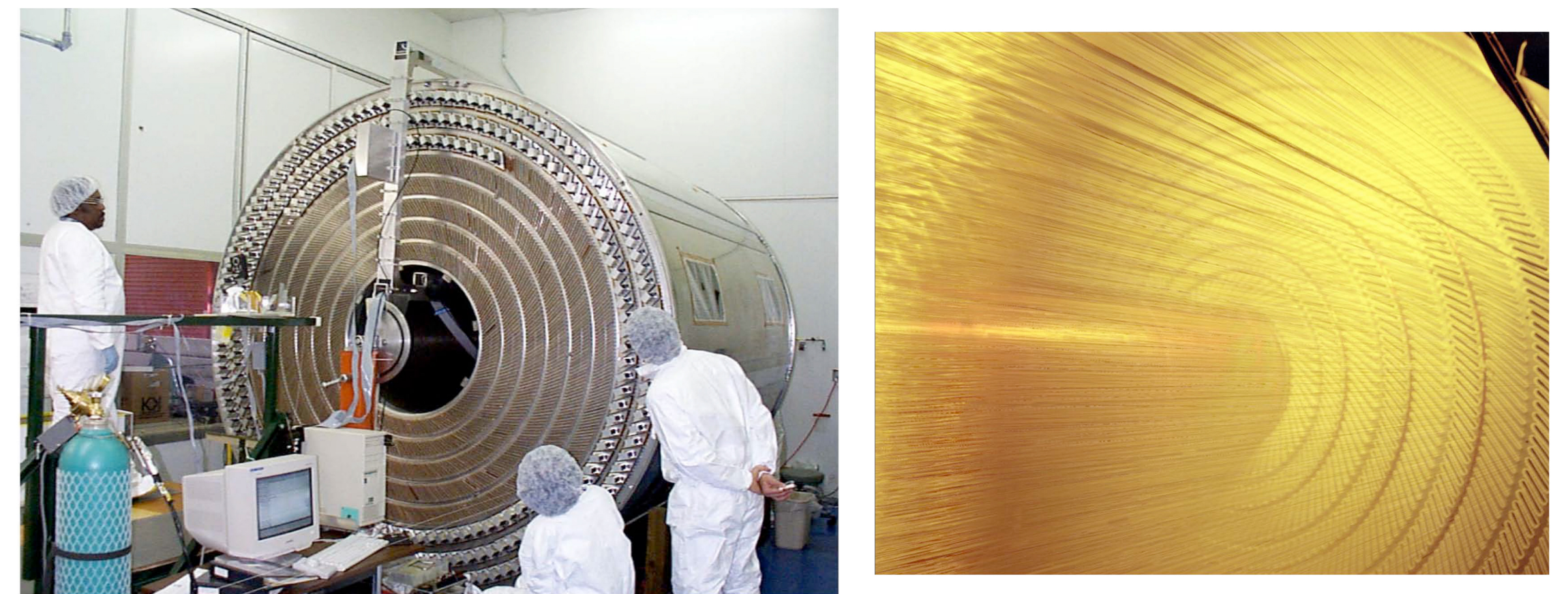
Figure 9.6: The central tracking detector of the CDF experiment at Fermilab's Tevatron..
