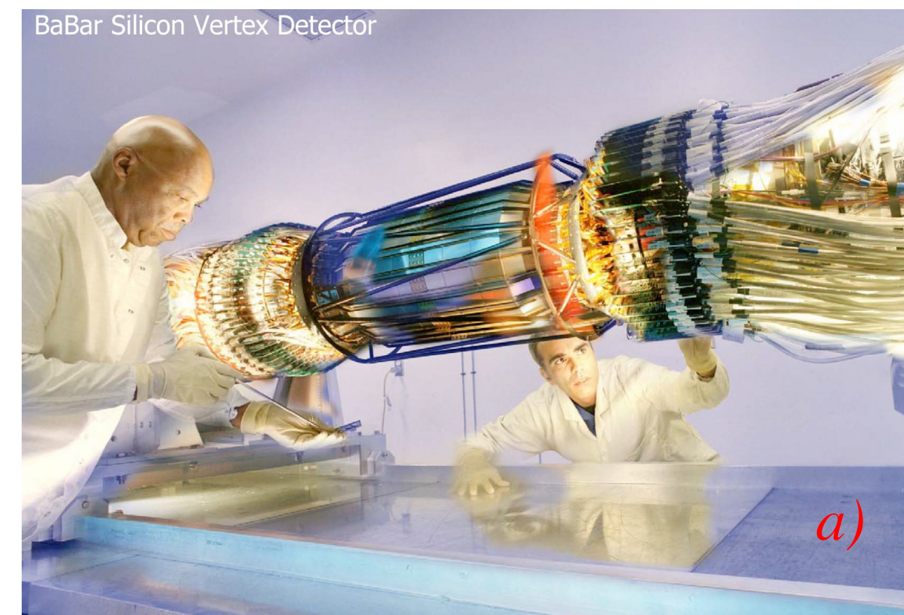
Figure 9.10: The Silicon Vertex Detector used in the BaBar experiment at SLAC. The insert shows the type of events that can be resolved with such instruments.
